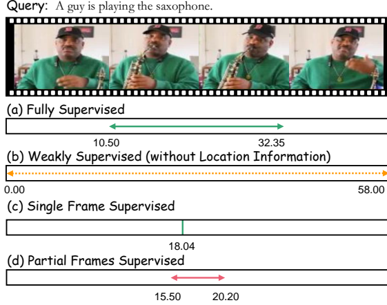
Figure 1: Illustration of Video Moment Retrieval tasks in different settings. The green arrow represents the supervision. (a) is fully supervised setting with precise temporal labels, such as timestamp of (10.50, 32.35); (b) is weakly supervised setting without any location information; (c) is single frame annotation as supervision, such as timestamp of (18.04). Compared with (a), (b), and (c), our proposed weak-supervised setting (d) provides partial location signals that are without controversy.
